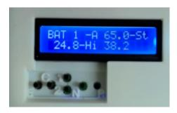
Press C to erase Data, and go back to Batch 1, the data is deleted on SD card (Confirmation is asked by pressing 1)
