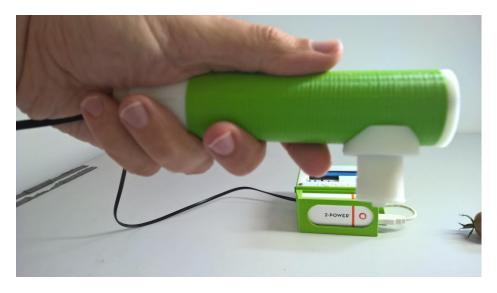
The devices takes the origin when you switch it on. If the sensor is not in the right position when you start the device, you can have a mistake in the measurements that can reach up to 60 grams
