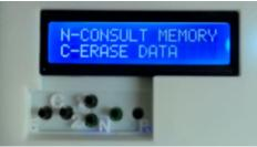
Press N for batched consultation – Each batch statistics is displayed during 3.5 seconds – "A" corresponds to the average, "St" is the standard deviation of the batch, "Hi" corresponds to the homogeneity index of the batch (shall be less than 10% for good homogeneity)
