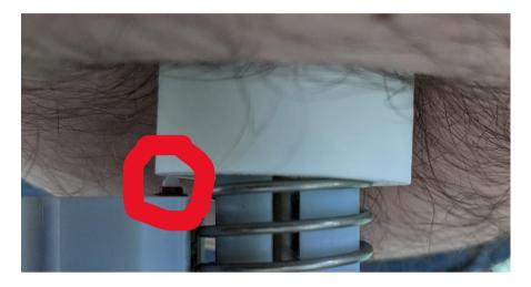
Press perpendicularly to the surface of the sample till the switch of the abutment is triggered. The device will make measurements each 70 milliseconds, and then stop once the abutment switch is triggered.
